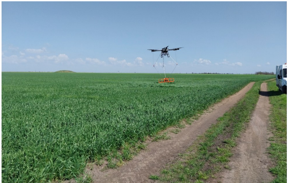
Figure 5. Surveying using the MinesEye system (Sensys R3 in drone-based GNSS mode mounted on extender).
