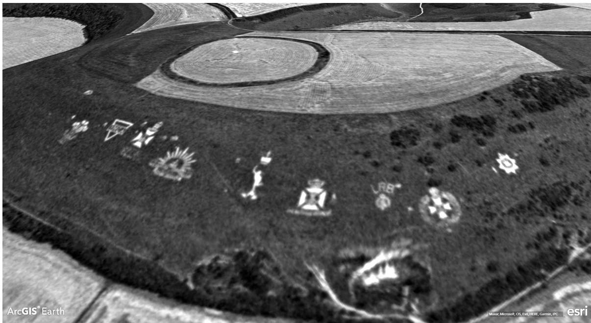
Figure 7. Extract from a KH-9 HEXAGON panoramic camera photograph the Fovant Badges, Wiltshire, georeferenced and draped over a digital elevation model using ArcGIS Earth. Image courtesy of the US Geological Survey. Entity ID: entity ID: D3C1206-300341F016.
